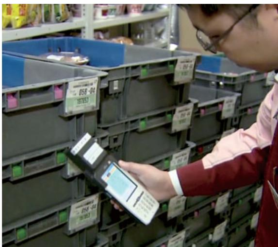
\*Radio-frequency identification (RFID) is a technology for contactless reading of data from an IC chip through the transmission of radio waves.
