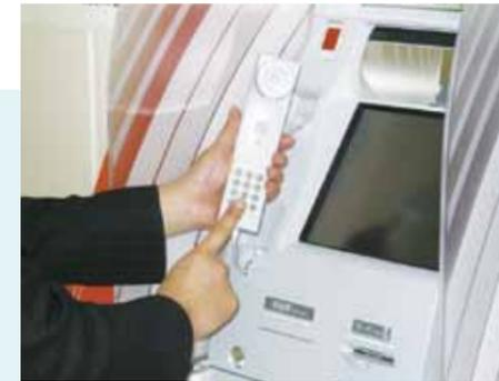
Transaction is completed with the intercom only, without using the touch panel.
