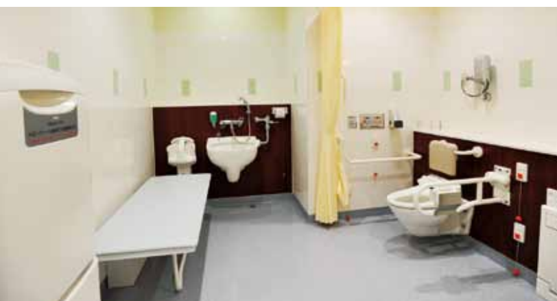
A multi-purpose toilet with a wide entrance, carefully laid out toilet seats and sink height, with voice guidance available. At Ario Hashimoto, two out of 12 restrooms may also accommodate ostomates.
