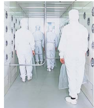
To maintain the production site dust and hair free, air shower and thorough hand washing is required before entering the room.
