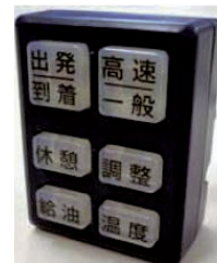
Six-buttoned device, recording departure and return from/to distribution centers
